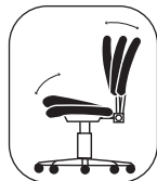
Seat & Back Multi-Knee Tilt/Lock Control Seat & back tilt together from a pivot point near the seat front, locking in various positions.
