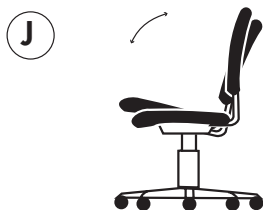
J Adjustable Tilt - Tension Control tension of seat can be increased or decreased as desired
