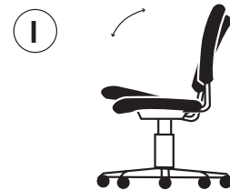
I Seat & Back Multi-Tilt Lock Control seat and back tilt together at the same angle, locking in an infinite number of positions
