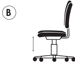
B Pneumatic Seat Height Control seat height can be increased or decreased
