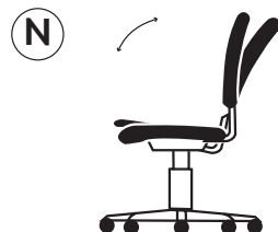
N Synchro-Tilt seat and back tilt together at a 2-1 ratio, for every 2 degrees of back recline the seat tilts 1 degree
