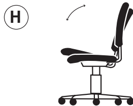
H Seat & Back Multi-Tilt seat and back tilt together at the same angle
