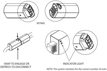
NO IE: I he system monitors for the correct number of units. Once connected to power, the light on control box will be green. If more than 8 Power/Data or Jumper units are plugged into the control box, power will shut down and light will be red.
