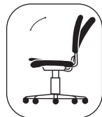
Synchro-Tilt Control Seat and back tilt together at a 2-1 ratio. For every 2 degrees of back recline, the seat tilts 1 degree.
